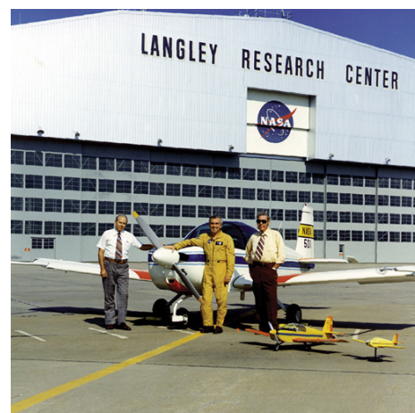
Above: James Patton Jr. (center) stands with James Bowman Jr. (left) and Sanger Burk (right) in front of a low-wing spin-research aircraft. A radio-controlled model and a spin-tunnel model of the same configuration are in the foreground. Credit: NASA.
