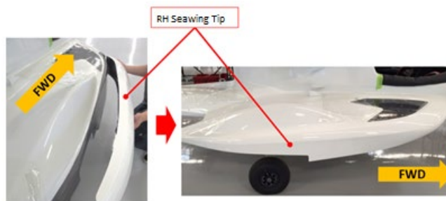
Figure 6 Seawing Tip Installation
