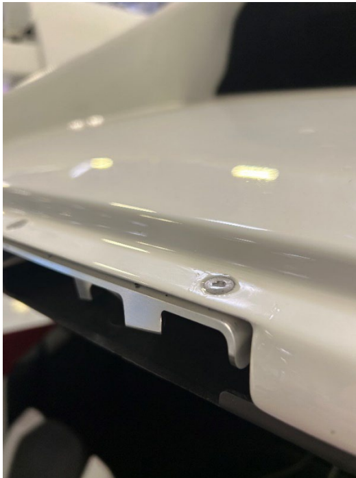
Figure 1. Sealant Applied Over Screw Heads
