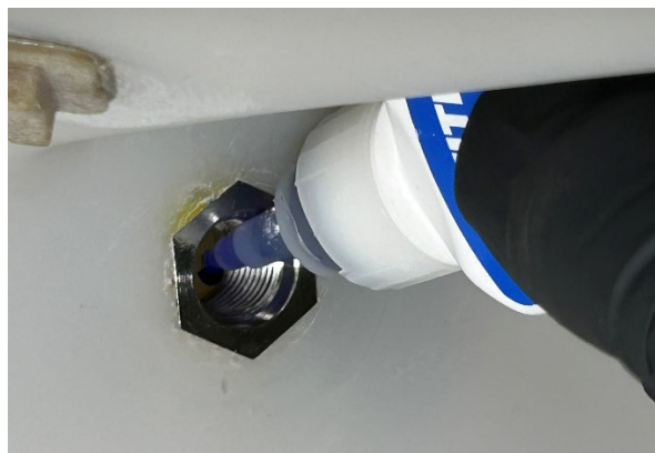
Figure 7. Apply ONE Drop of Loctite 425 to the Middle of the Insert
